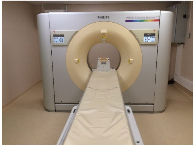
Figure 1. Prototype pre-clinical photon counting x-ray CT system used for measurements.
